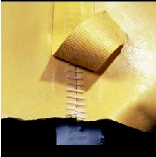
**TRELLCHEM HPS/VPS SEAM** Stiched with aramide thread for superior strength and durability. Taped with a rubber strip on the outside and a barrier laminate strip welded to the inside. This provides a continuous barrier layer across the seam.
